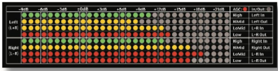
Using the '0dB' column of LEDs as reference or unity gain (10 LEDs in each horizontal row being lit), more LEDs to the right indicate greater than unity gain, and fewer LEDs lit indicate less than unity gain.
