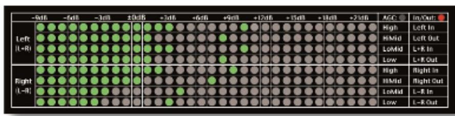
RMS (average) levels are indicated with a solid bar of green LEDs from the left, and the peak level is indicated with a single LED to the right of the RMS level. A 'peak stretch' feature to allow you to more easily see brief peaks by holding the LED at peak level momentarily.
